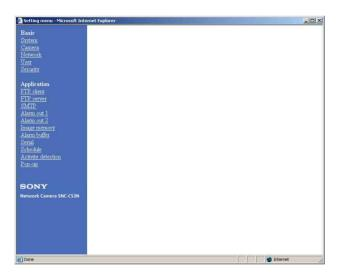
The Administrator menu consists of the Basic menu and the Application menu. The Basic menu is used for basic settings of the camera, and the Application menu is used for setting various applications according to individual. Click on each menu name to display its setting page.
